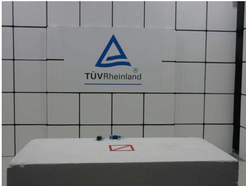
Photograph 3: Set-up for Radiated Emission (above 1 GHz)
