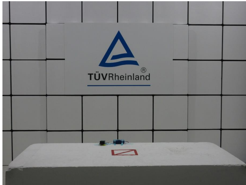
Photograph 2: Set-up for Radiated Emission (up to 1 GHz)
