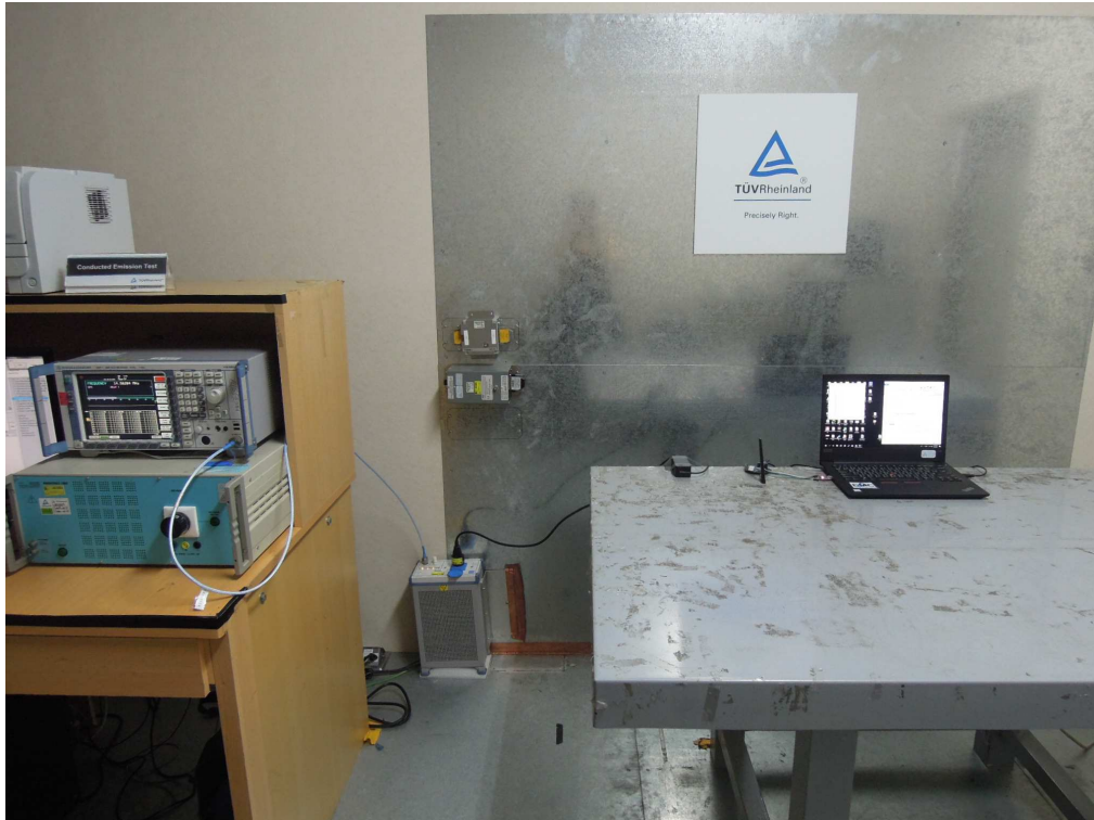
Photograph 7: Set-up for for Mains Conducted testing Front
