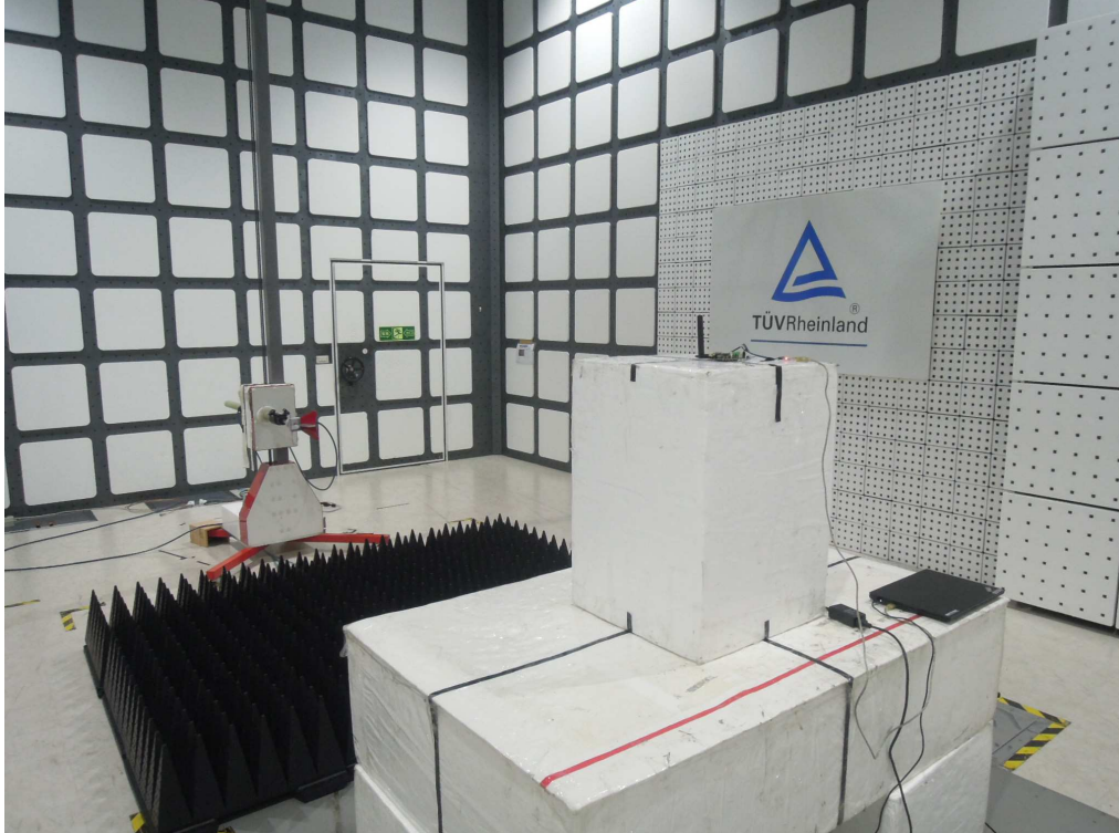
Photograph 3: Set-up for Spurious Emissions (Back View 2)
