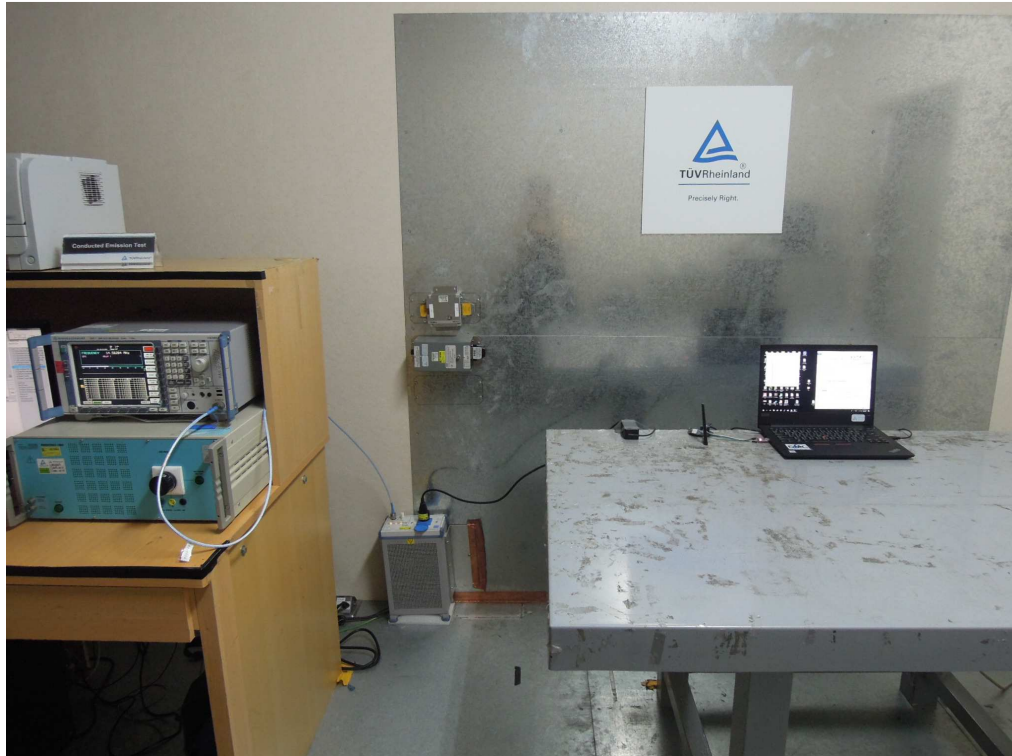
Photograph 7: Set-up for for Mains Conducted testing Front
