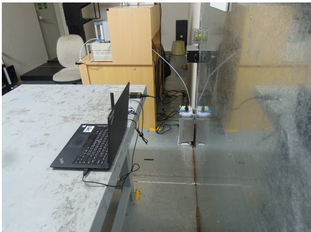
Photograph 6: Set-up for for Mains Conducted testing Back
