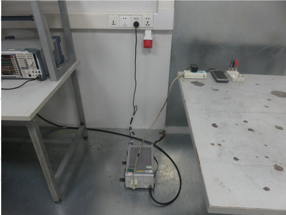
Photo of Conducted Emission Measurement
