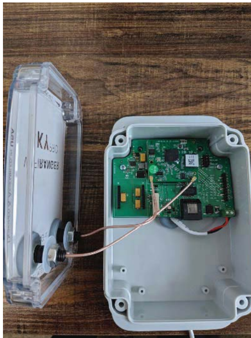
Figure : Assembled with Two 0dBi 2.4GHz Antennas connected to WiFi module.
