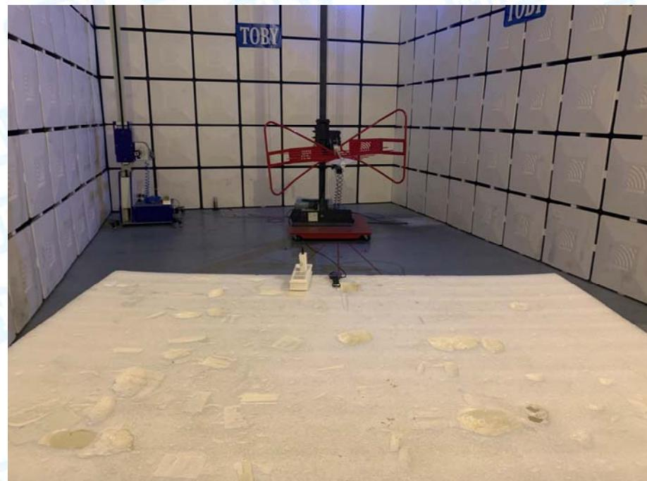
**Photo of Setup for Conducted Emission**
