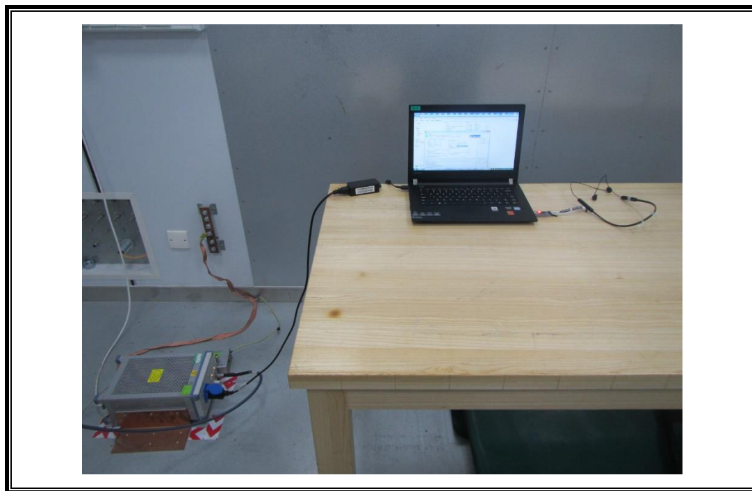
POWERLINE CONDUCTED EMISSIONS MEASUREMENT SETUP
