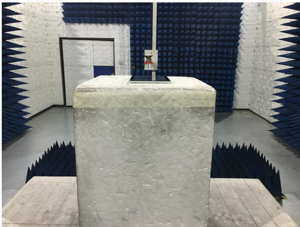
FCC RADIATED EMISSION TEST SETUP ABOVE 1GHZ
