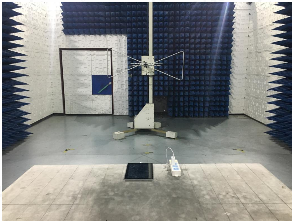
FCC RADIATED EMISSION TEST SETUP ABOVE 1GHZ
