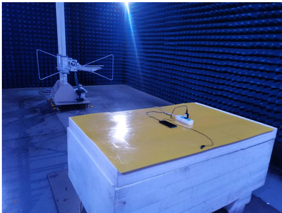
Photo of Radiated Emission Measurement (Above 1G)
