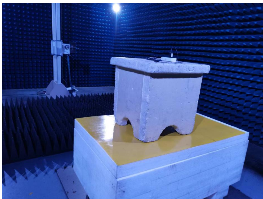
Photo of Radiated Emission Measurement (Above 1G)
