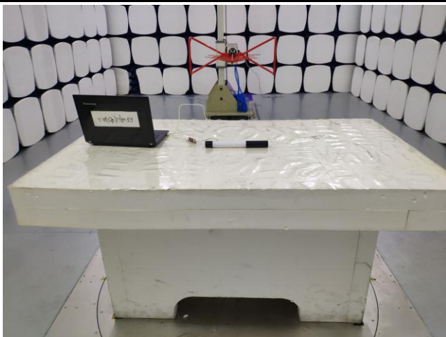
Conducted Emissions Test Setup Front View
