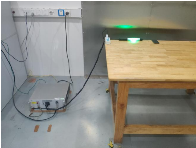
Conducted Emissions Test Setup Front View
