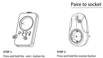
Press and hold the receiver button 3 secs to activate the remote control for 3 secs, the red LED blinks indicating pairing mode. The icon **CONNECT** flashes the socket is in pairing mode.
