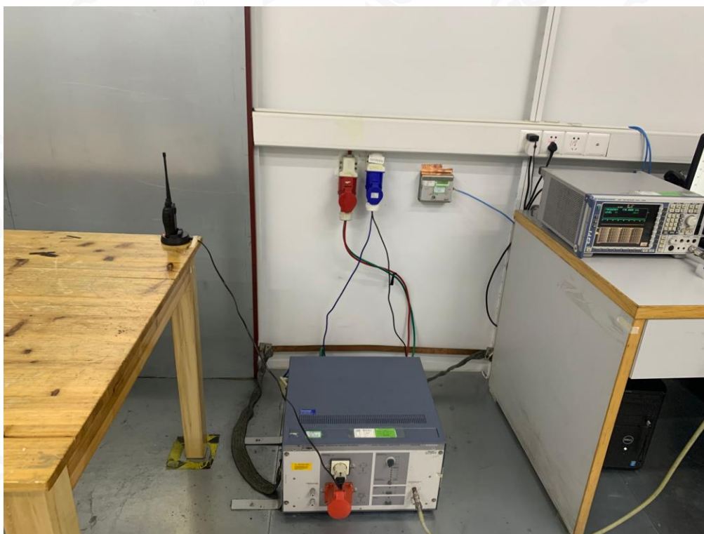
RADIATED EMISSION TEST SETUP-BELOW 1GHZ
