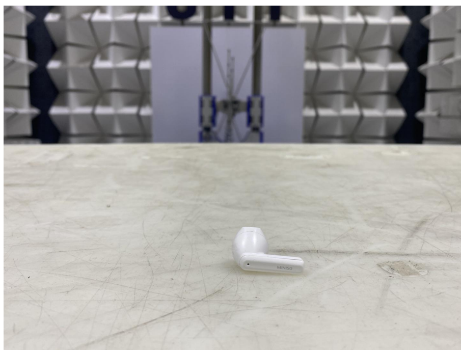
Radiated spurious emission Test Setup-2(Below 1GHz) Close-up
