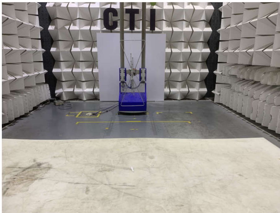
Radiated spurious emission Test Setup-1 left ear(Below 1GHz)
