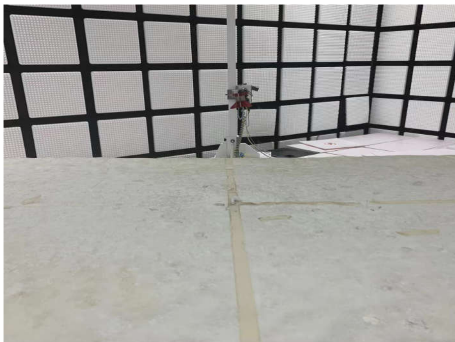
Radiated spurious emission Test Setup-2 left ear(Above 1GHz)
