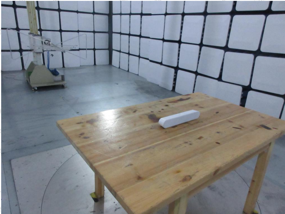
Photo of Radiation Emission Test
