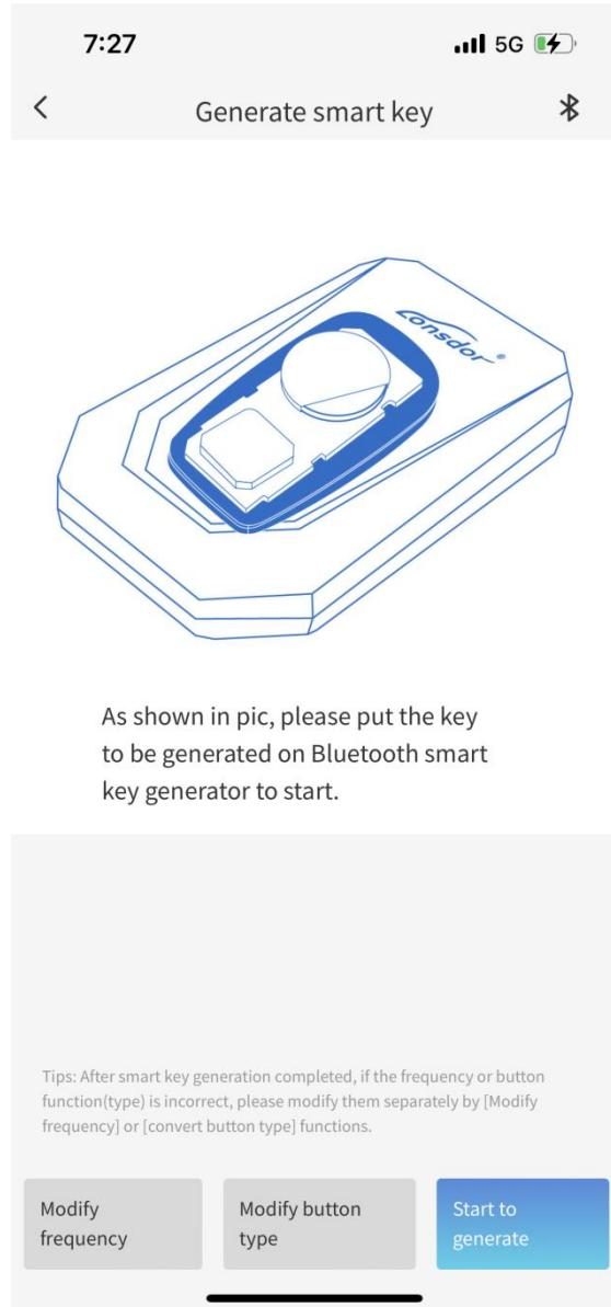
Click More Functions to Get version information, Read button function, Modify button type, Modify frequency, Generate smart key, Upgrade key, Modify remote count value, Unlock key, etc.
