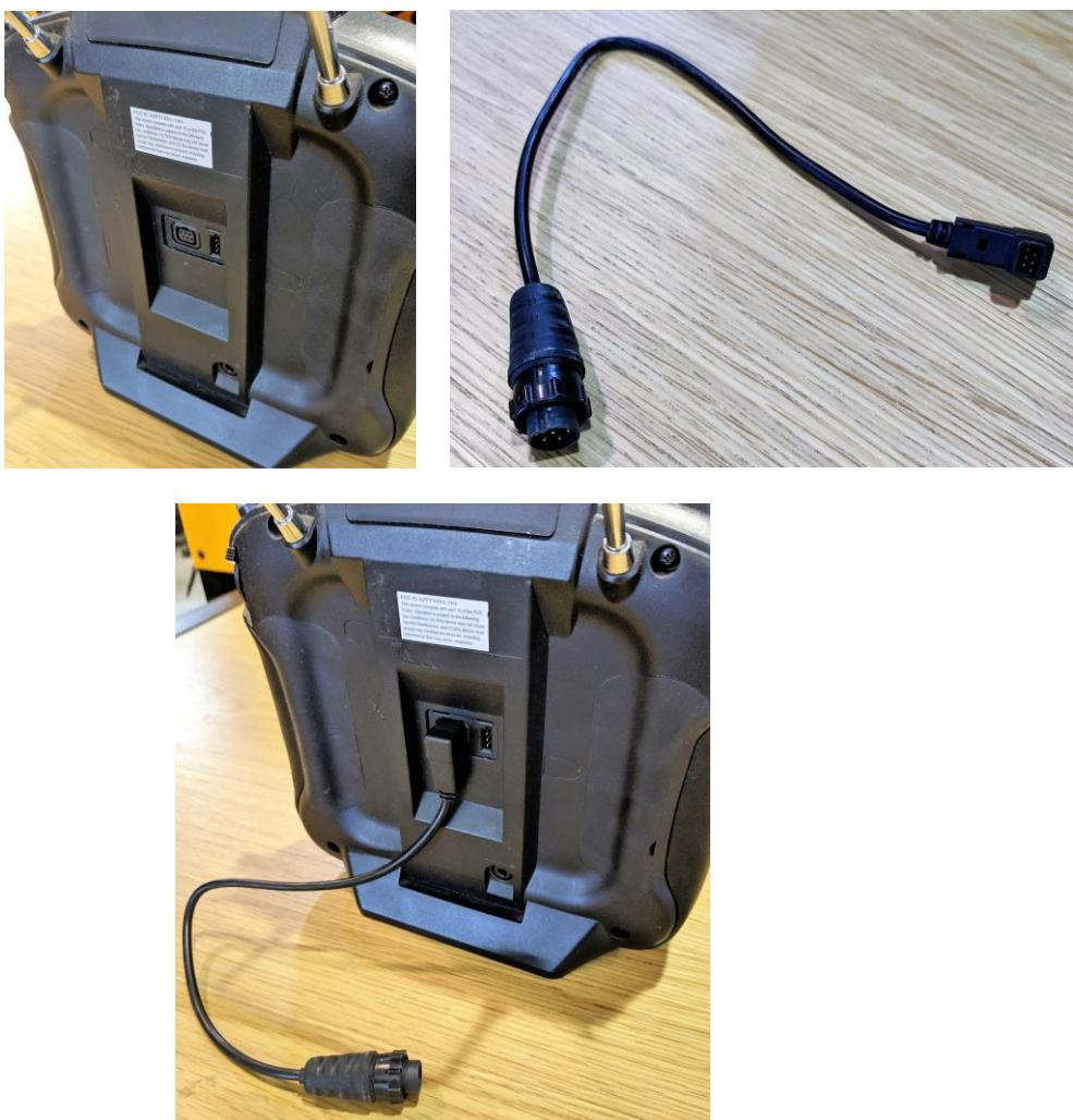
4. Connect the trainer cable to the LoRa module
