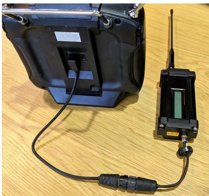
5. Connect the battery to the LoRa module, this will power up the AO00059 and will start transmitting the remote-control trainer output.
