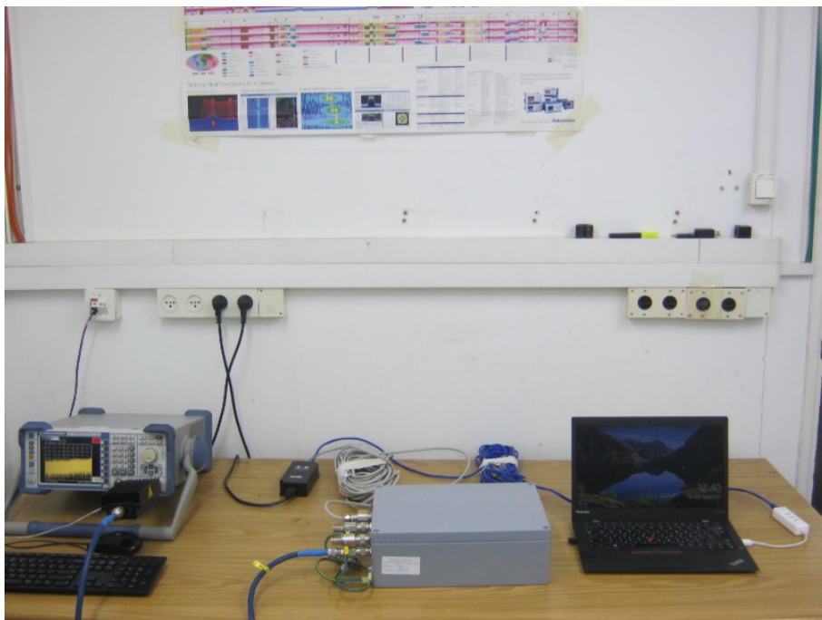
Figure 4. Conducted Emission Test
