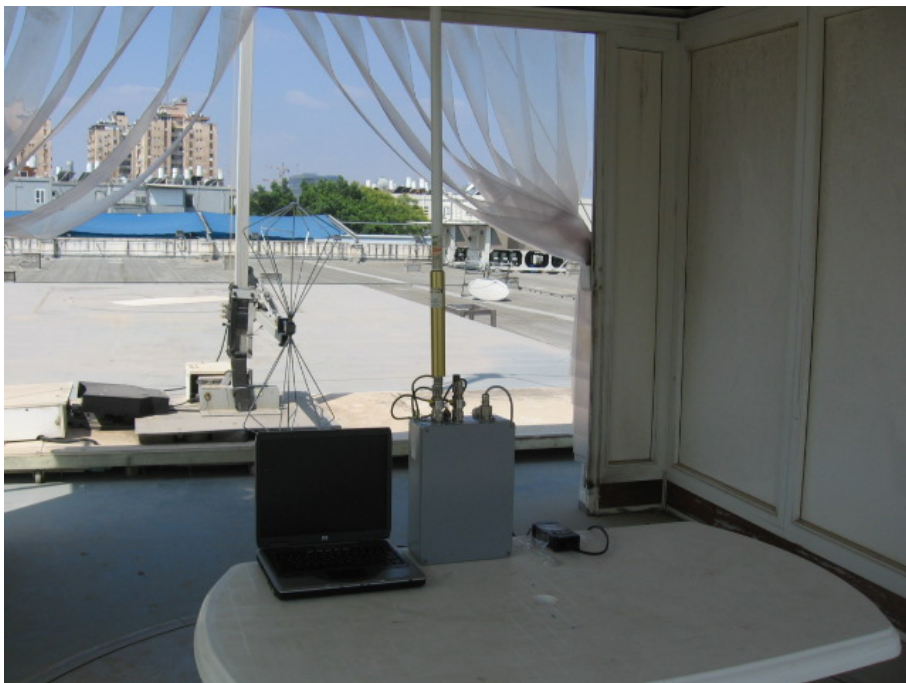
Figure 6. Radiated Emission Test, 30-200MHz
