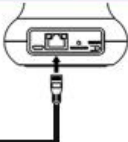
1. Connect the cable to the router and camera as shown in the picture
