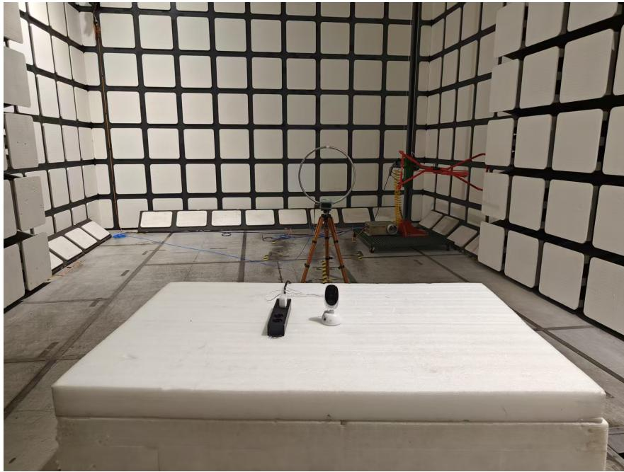
**Radiated Emissions View (30 MHz- 1 GHz) (Adapter 2: EP04-050100WXLZ)**
