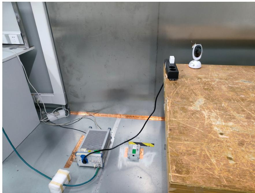
**Conducted Emissions - Side View (Adapter 1: AT-538A-050100A)**
