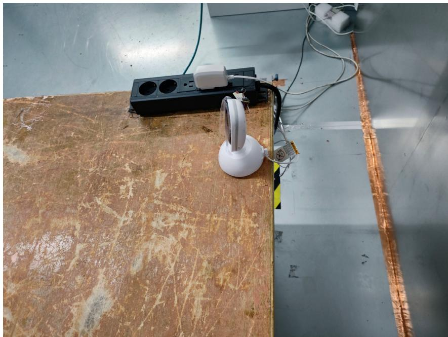
**Radiated Emissions View (9 kHz- 30MHz) (Adapter 1: AT-538A-050100A)**
