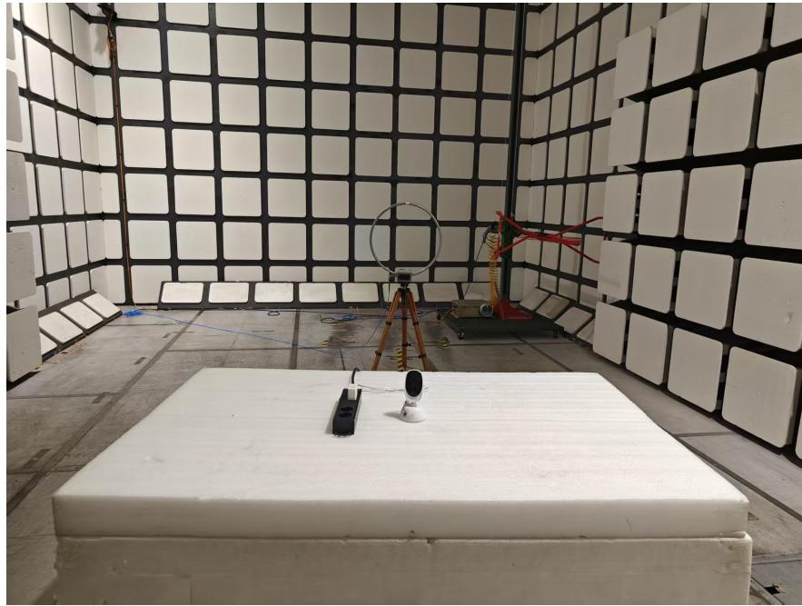
**Radiated Emissions View (30 MHz- 1 GHz) (Adapter 1: AT-538A-050100A)**
