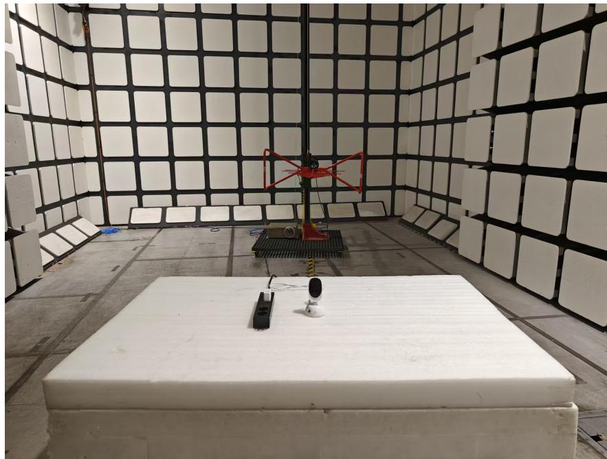
**Radiated Emissions View (9 kHz- 30 MHz) (Adapter 2: EP04-050100WXLZ)**
