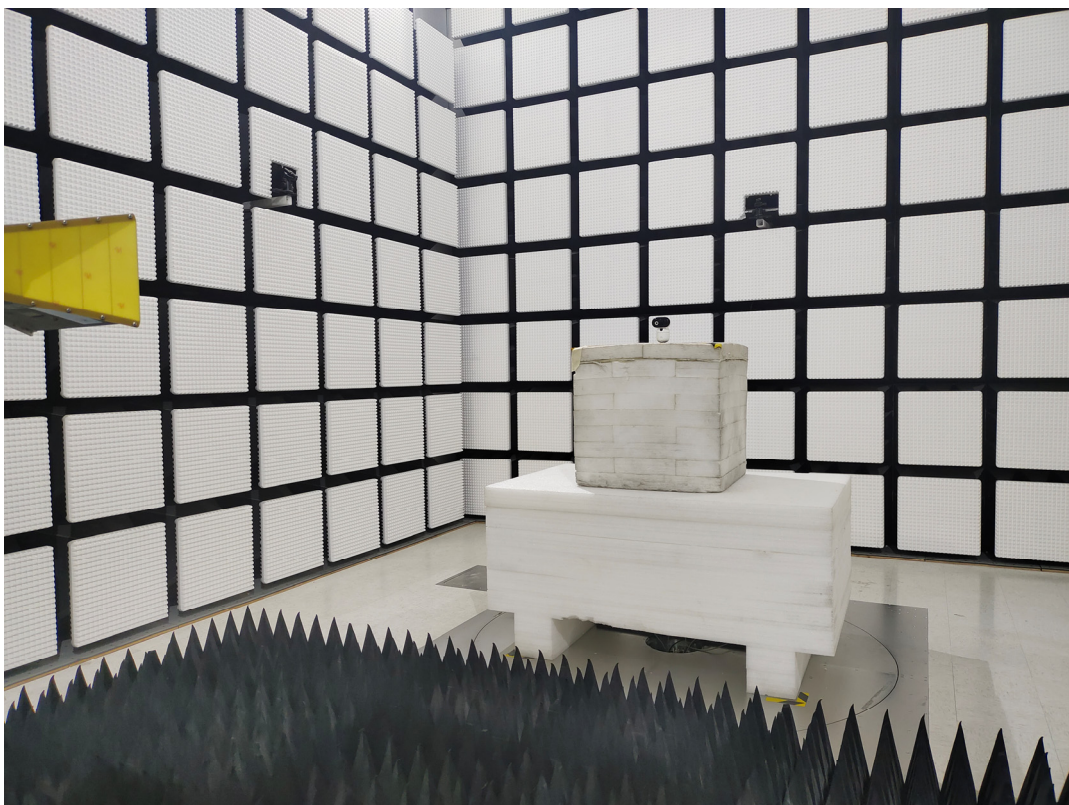
Radiated Emission Above 1GHz View
