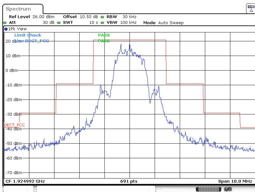
**High Channel (Unwanted Emission inside the Sub-band)**
