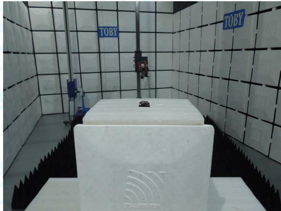
**Photo of Setup for Radiated Emission (Below 1 GHz)**
