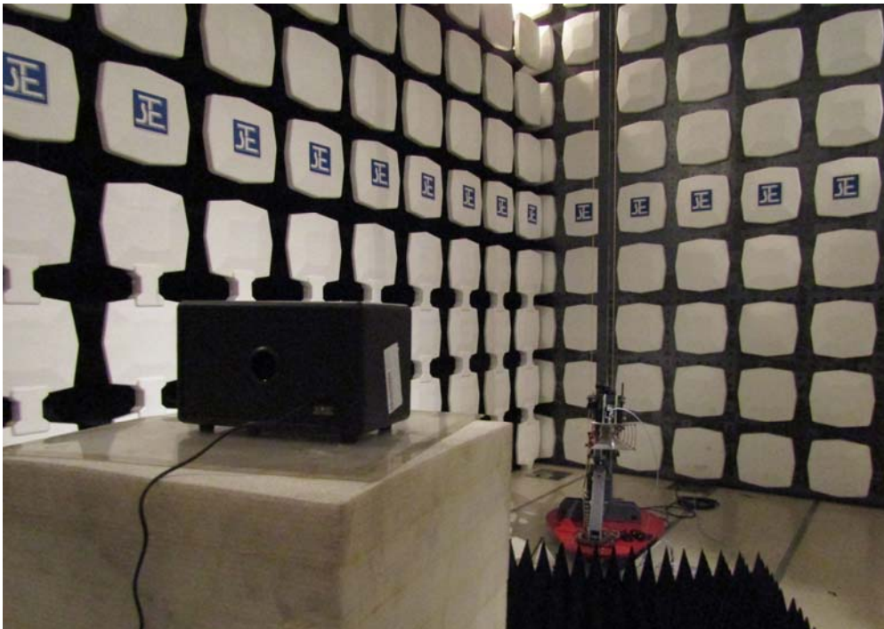
Measurement of Radiated Emission Test Set Up
