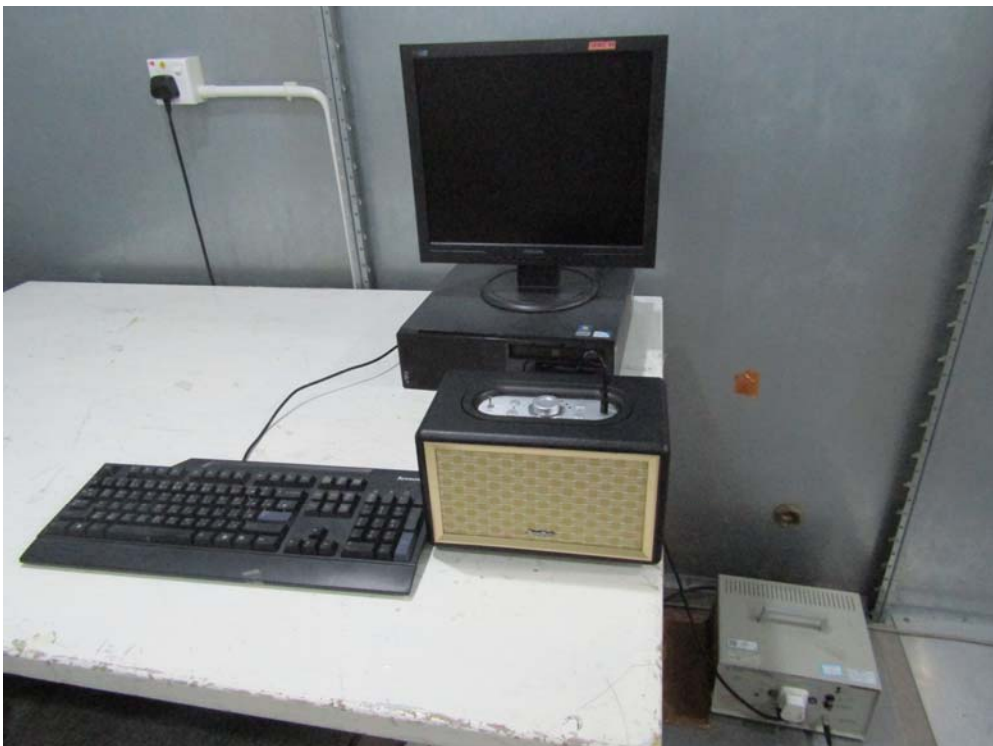
Measurement of Conducted Emission Test Set Up
