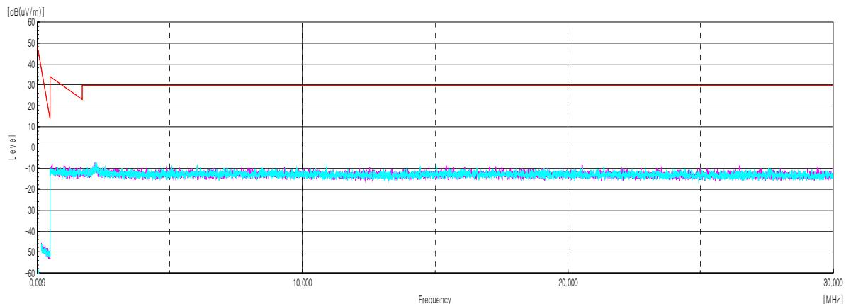
**Test results (Below 1 000 MHz) - Field strength of fundamental**
