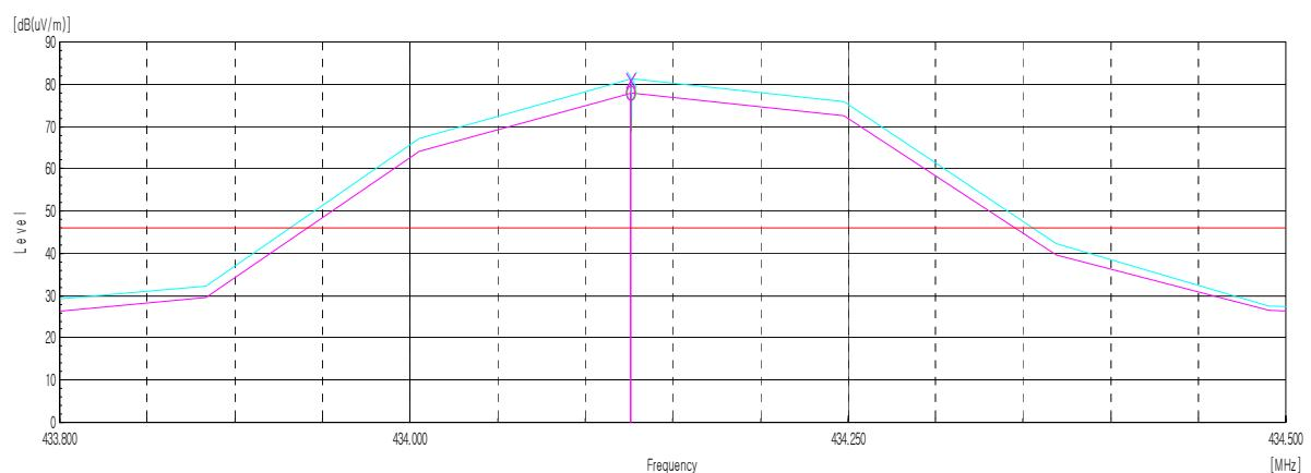
**Test results (Below 1 000 MHz) – Spurious emission****Low Channel**
