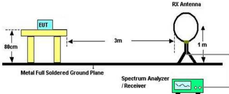
The setting of the spectrum analyzer
