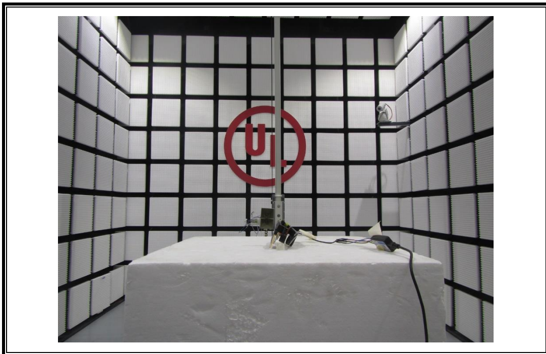
RADIATED RF MEASUREMENT SETUP (Y Axis)
