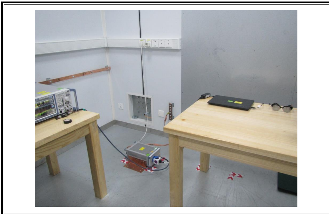
POWERLINE CONDUCTED EMISSIONS MEASUREMENT SETUP
