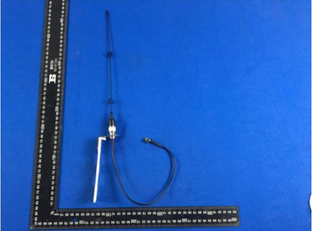
A photograph of the new LTE antenna assembly. It features a vertical black whip antenna mounted on a black base, connected to a black cable that loops back to a white connector. A black measuring tape is placed vertically next to the antenna for scale. |
