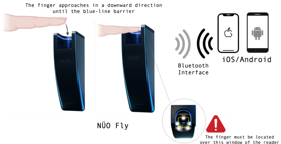
Figure 4. Operational description of NÜO FLY1 reader.
