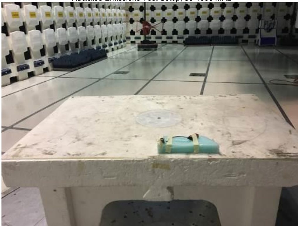
Radiated Emissions Test Setup, 30-1000 MHz
