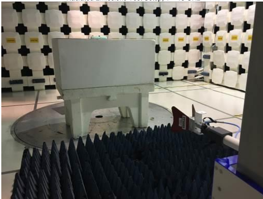
Radiated Emissions Test Setup, 1 – 18 GHz
