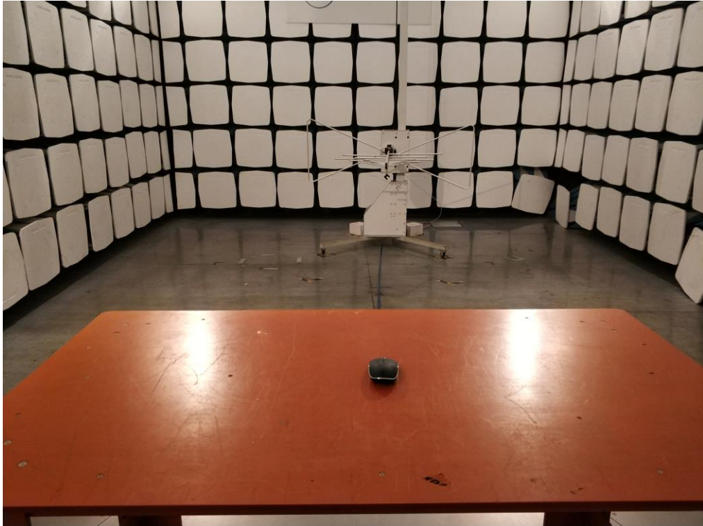
Radiated Emission Test
