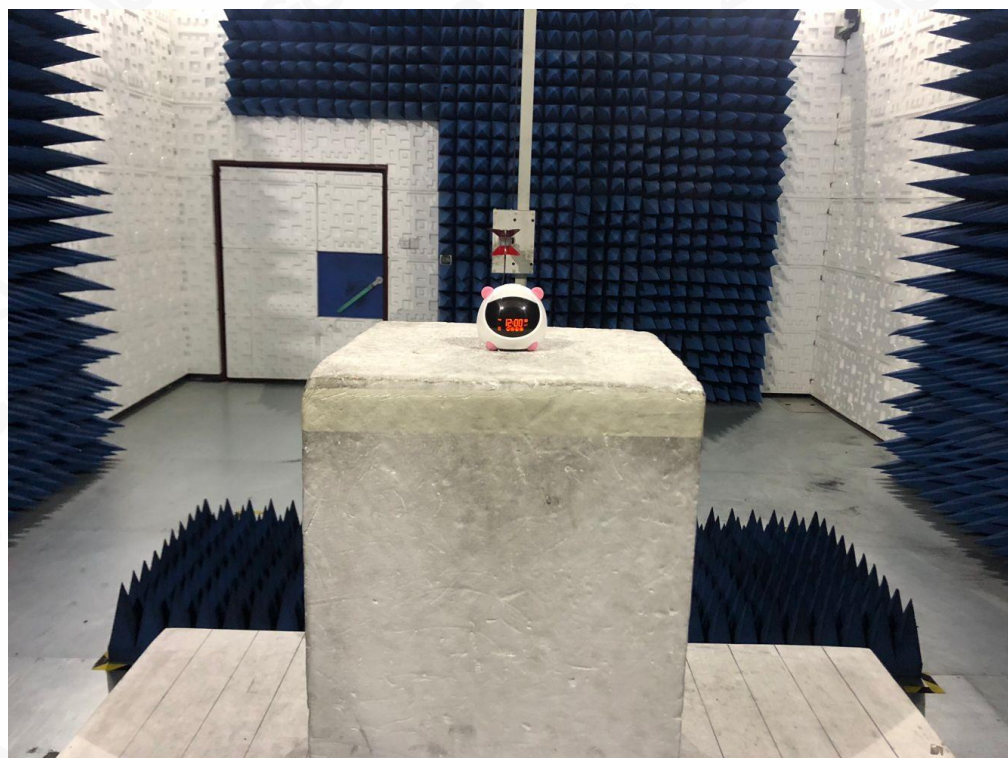
FCC RADIATED EMISSION TEST SETUP ABOVE 1GHZ
