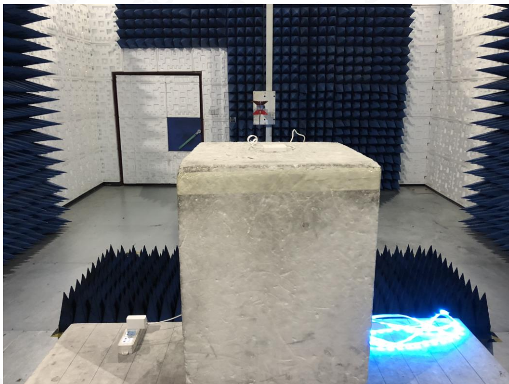
FCC RADIATED EMISSION TEST SETUP ABOVE 1GHZ
