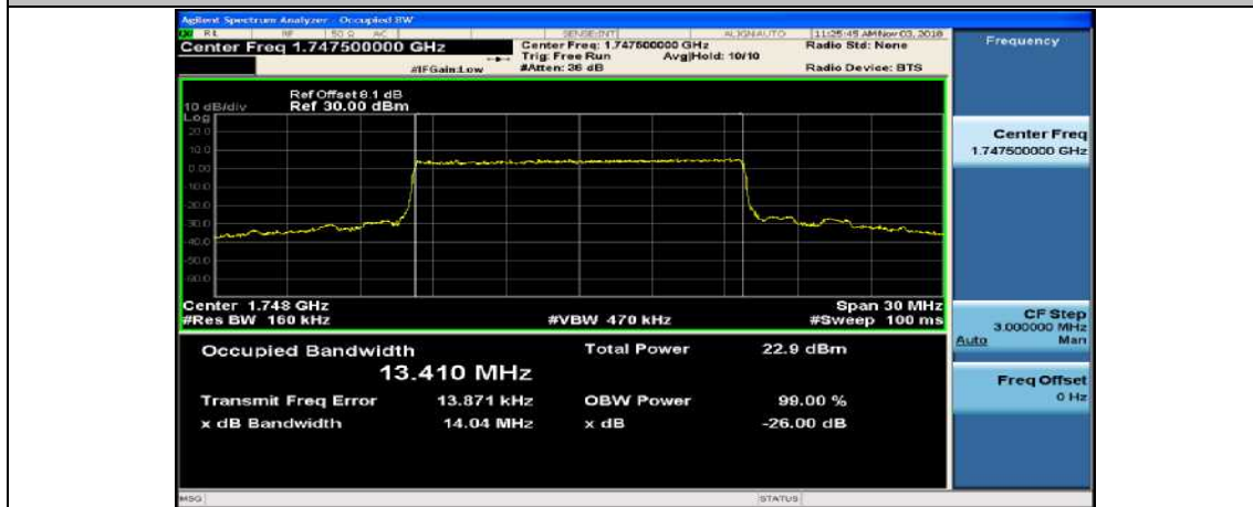
(Channel Bandwidth:15 MHz)_HCH_QPSK_75RB#0
