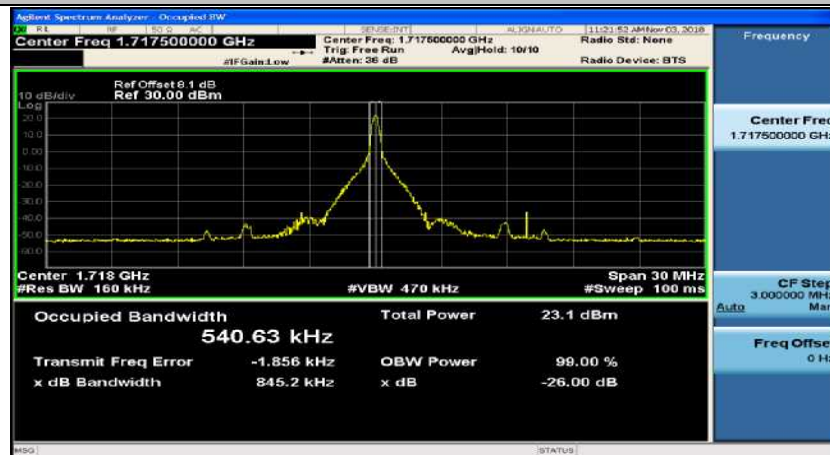
(Channel Bandwidth:15 MHz)_LCH_16QAM_1RB#74
