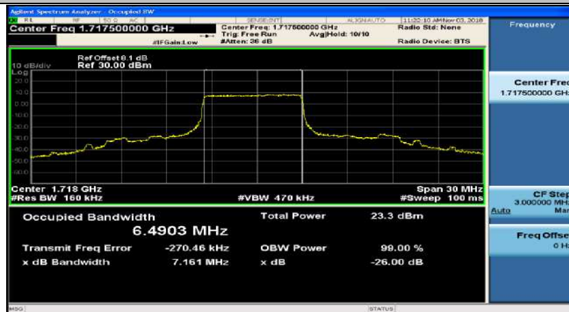
(Channel Bandwidth:15 MHz)_LCH_QPSK_37RB#38
