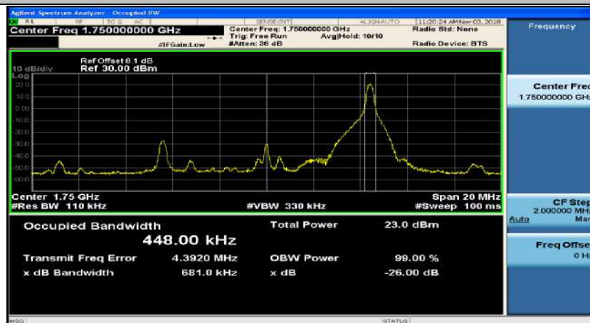
Channel Bandwidth: 10 MHz_HCH_16QAM_1RB#49
