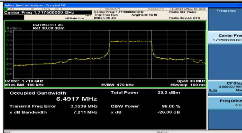
(Channel Bandwidth:15 MHz)_LCH_QPSK_37RB#38
