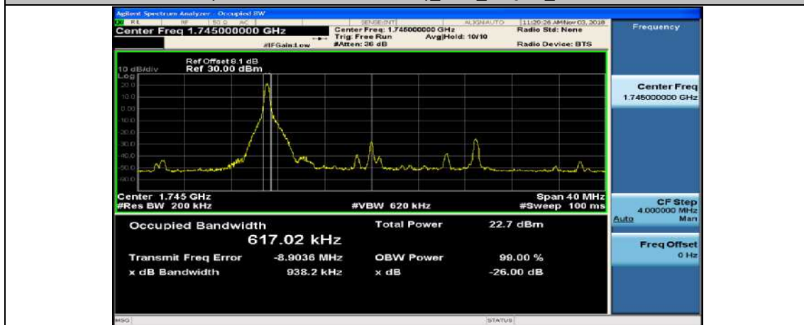
(Channel Bandwidth:20 MHz)_HCH_16QAM_1RB#50
