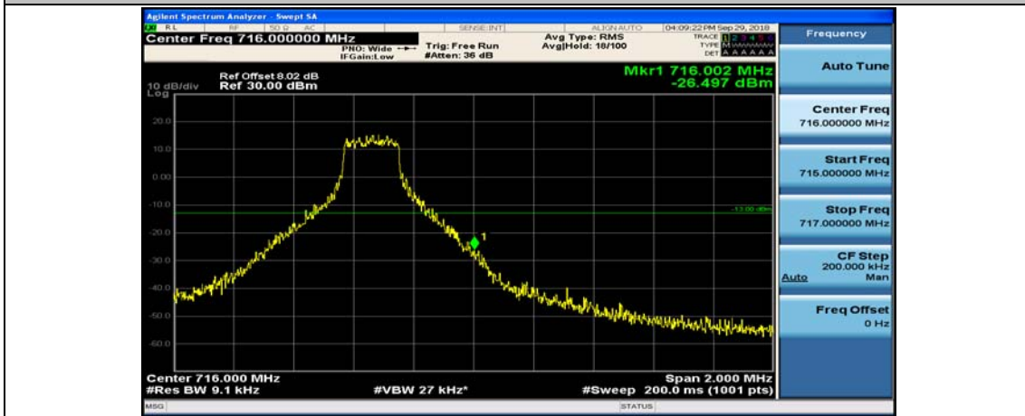
(Channel Bandwidth: 5 MHz)_HCH_16QAM_12RB#0
