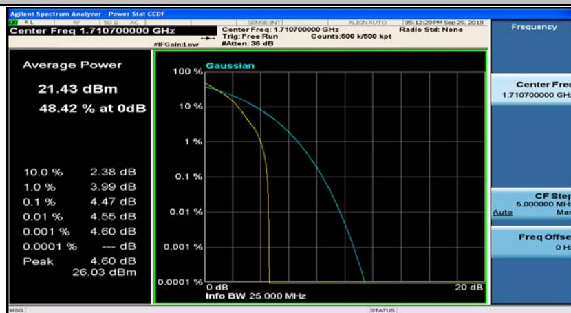
(Channel Bandwidth: 1.4 MHz)_LCH_QPSK_3RB#0
