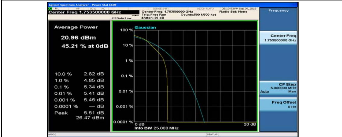
(Channel Bandwidth: 3 MHz)_HCH_16QAM_1RB#7
