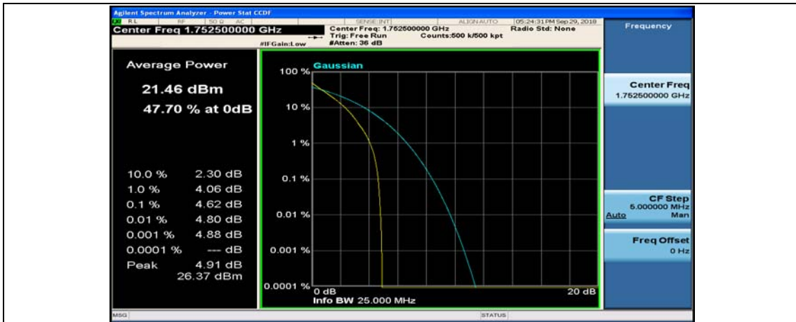
(Channel Bandwidth: 5 MHz)_HCH_QPSK_12RB#13
