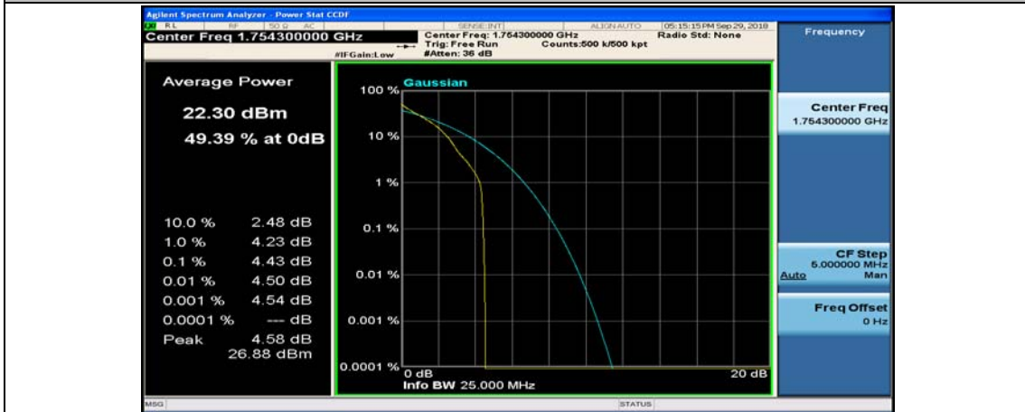
(Channel Bandwidth: 1.4 MHz)_HCH_QPSK_1RB#3
