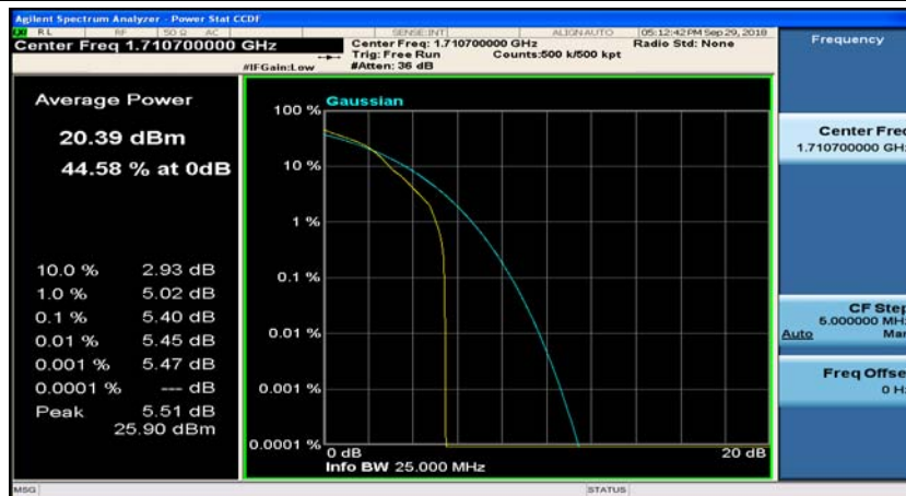
(Channel Bandwidth: 1.4 MHz)_LCH_16QAM_1RB#5
