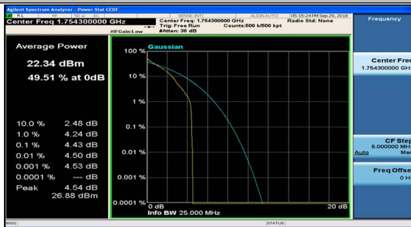
(Channel Bandwidth: 1.4 MHz)_HCH_QPSK_3RB#0
