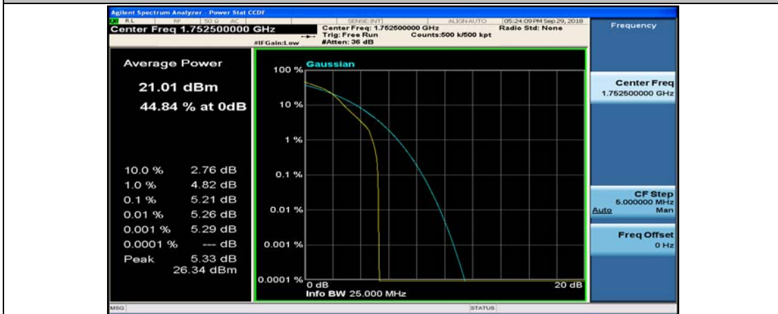
(Channel Bandwidth: 5 MHz)_HCH_16QAM_1RB#12
