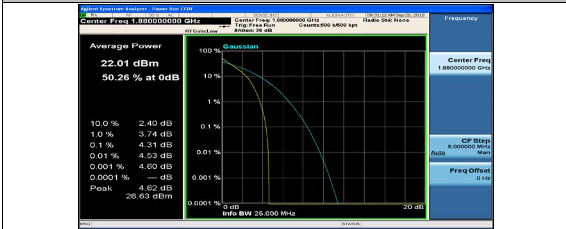
(Channel Bandwidth: 3 MHz)_MCH_QPSK_15RB#0
