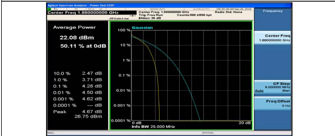
(Channel Bandwidth: 3 MHz)_MCH_QPSK_8RB#4
