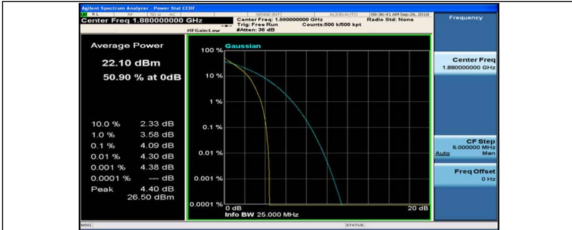
(Channel Bandwidth: 5 MHz)_MCH_QPSK_25RB#0
