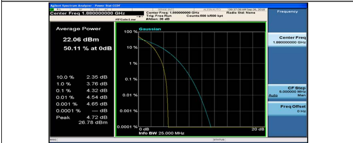
(Channel Bandwidth: 5 MHz)_MCH_QPSK_25RB#0
