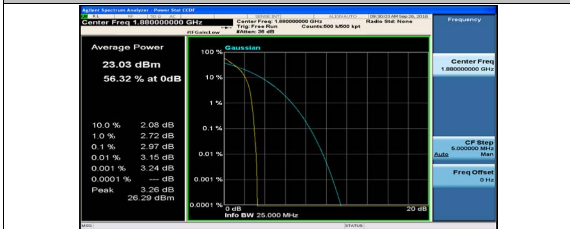
(Channel Bandwidth: 3 MHz)_MCH_QPSK_1RB#7
