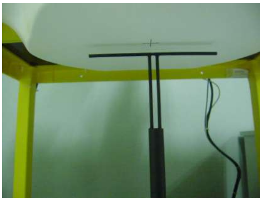
Setup Photo of Dipole Antenna
