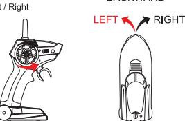
3. The navigation rudder can correct the navigation direction. When forwarding, you can manually adjust it to the left if it yaw right, or you can adjust it to the right if it yaw left.
