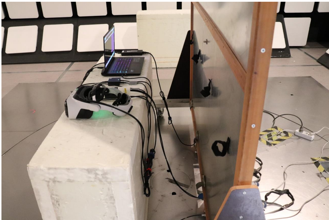
Photograph 2. Test setup for AC Power-Line Conducted Emissions
