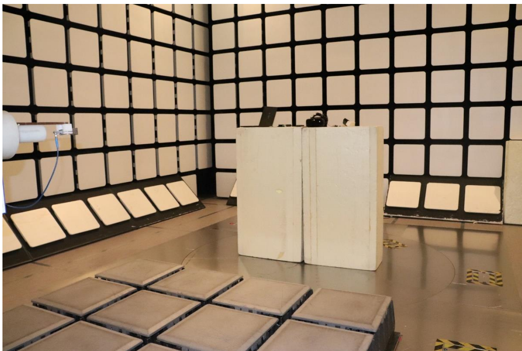
Photograph 5: Radiated emission test setup 18 GHz – 26.5 GHz
