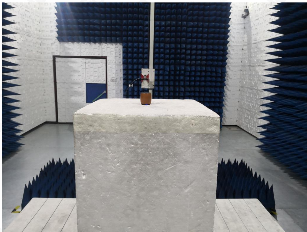
RADIATED EMISSION TEST SETUP ABOVE 1GHZ
