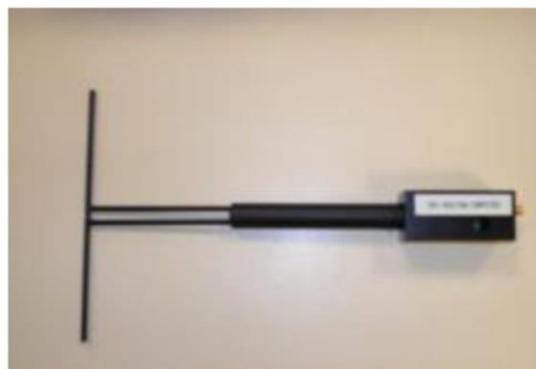
Figure 1 – Satimo COMOSAR Validation Dipole
