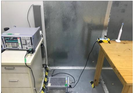
Radiated Spurious Emissions Test Frequency From 9kHz-30MHz
