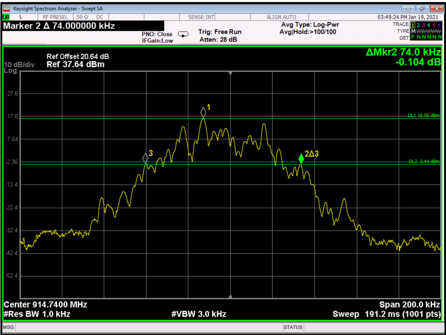
Figure 8 - 914.74 MHz – Emission Bandwidth
