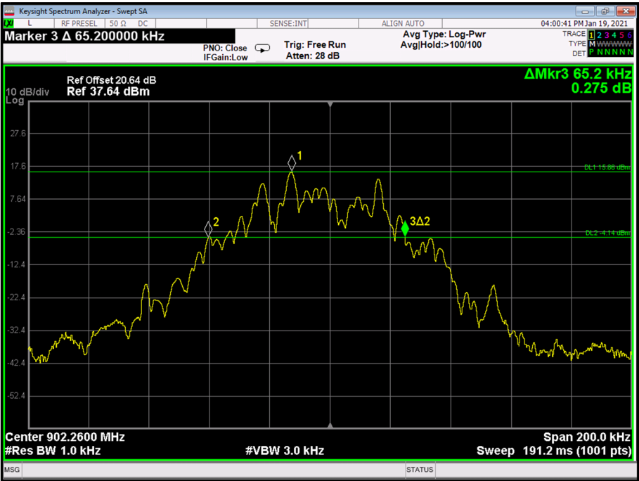
Figure 7 - 902.26 MHz – Emission Bandwidth
