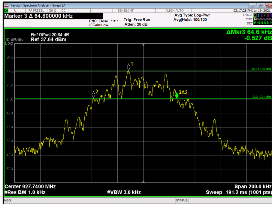
Figure 9 - 927.74 MHz – Emission Bandwidth
