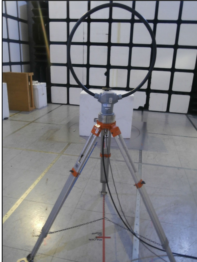
Figure 11 - Field Strength of Emissions - 150 kHz to 30 MHz
