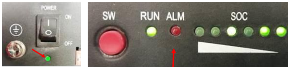
Figure 13: LEDs on Battery front panel indicating charging
