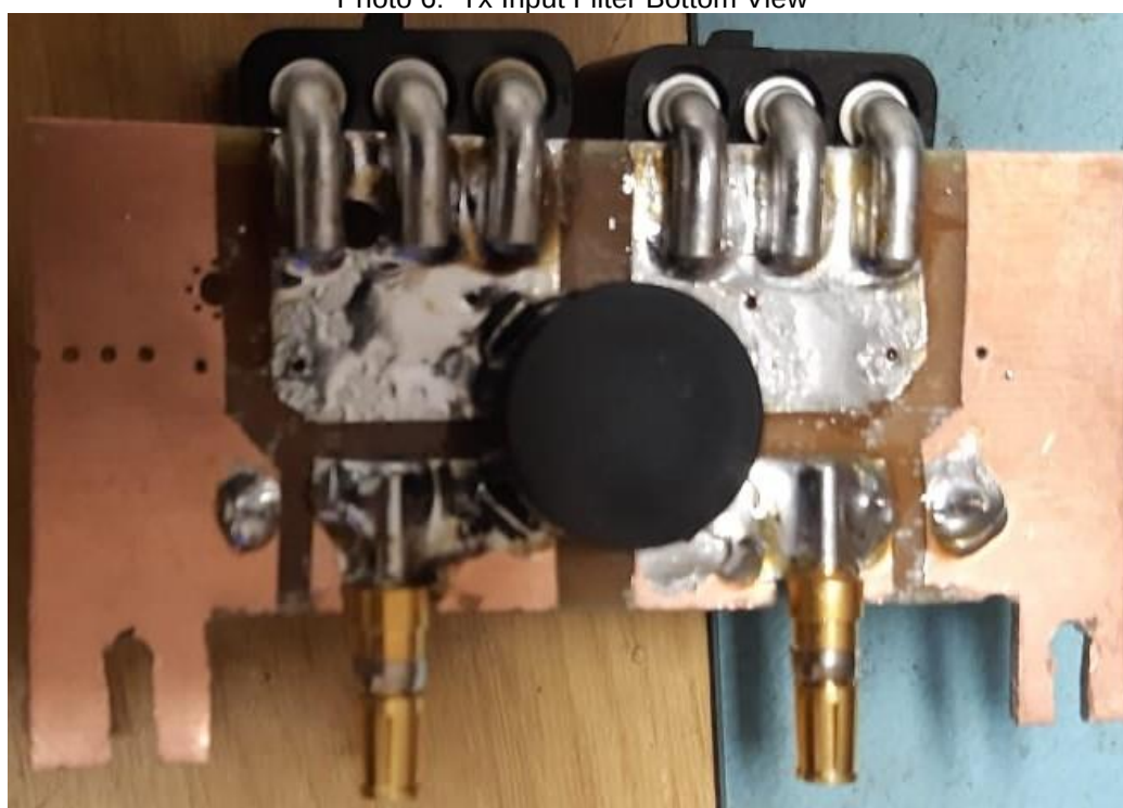
Photo 6: Tx Input Filter Bottom View
