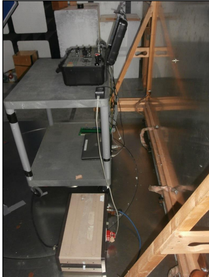
Figure 11 – Conducted Disturbance at Mains Terminals
