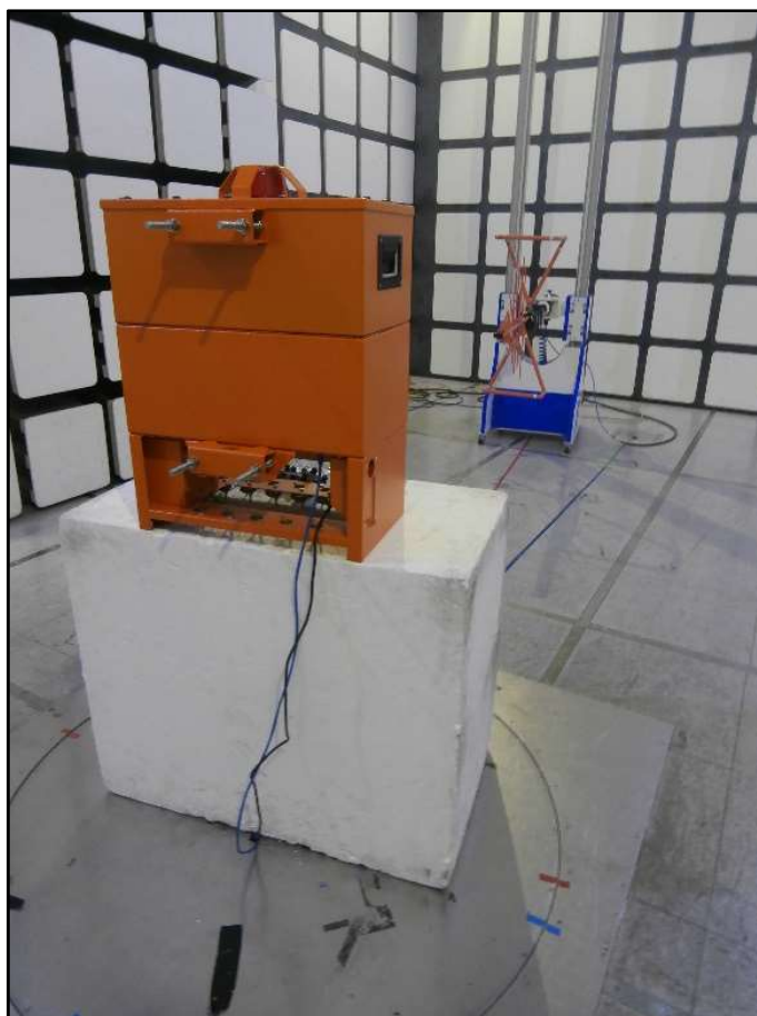
Figure 12 – Radiated Disturbance (30 MHz to 1 GHz)
