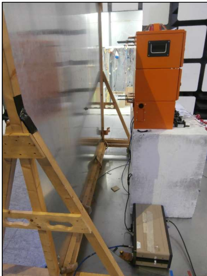
Figure 11 – Conducted Disturbance at Mains Terminals
